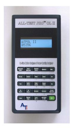
The ALL-TEST PRO On-Line II™ (ATPOL II™) tester is the ideal and most complete power diagnostic and energized motor instrument available! It is hand held, lightweight, and comfortable with its rubberized bottom for grip. There is no need to carry other heavy equipment around with you in the field.
