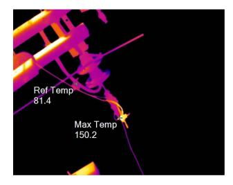
**Comments:** This left side line has a hot clamp connection defect. It has been reported on multiple times and has continued to increase in temperature.
